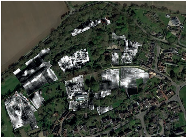
Fig.9 Plot of the completed resistivity survey overlain upon a GoogleEarth image (courtesy GoogleEarth)
